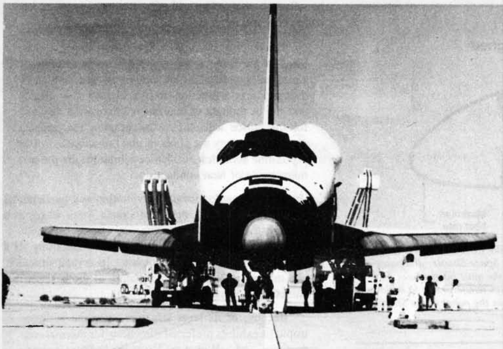
Vought Corp.'s Reinforced Carbon-Carbon, a gray material, protects the Space Shuttle's nosecap and leading edges of its wings.
