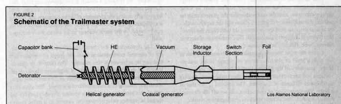
Trailmaster was conceived as a method to convert the cheap chemical energy of high explosives into compressed, high-power electrical pulses. This is achieved in two distinct stages. First, the chemical explosive energy is transformed into a pulse of electric current. Second, this pulse is compressed 100-fold, through utilizing fast-opening switches in a series of electrical circuits.
