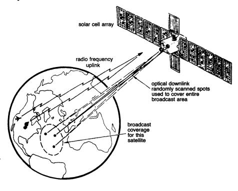
The Satellite Laser Communications system will transmit messages for submerged U.S. submarines to obtaining satellites via radio communications. The satellites will then transmit to the subs via flashes of blue-green laser light.
