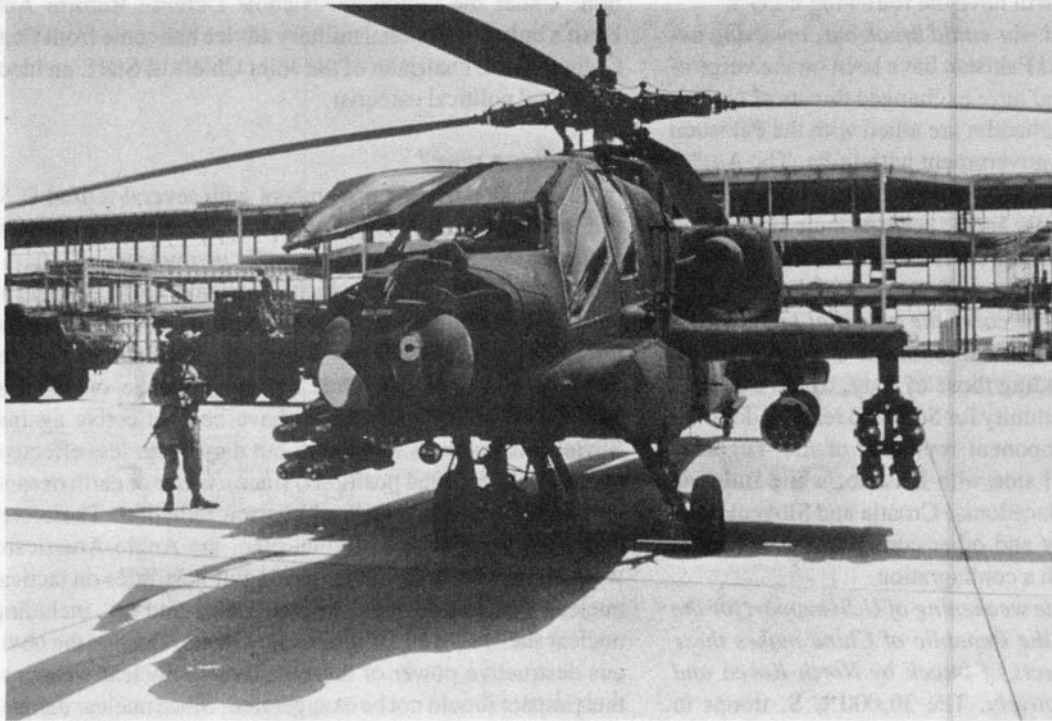
Soldiers of the U.S. 101st Airborne Division load ammunition on an AH-64 Apache helicopter in Saudi Arabia. The Apache, which would be a centerpiece of U.S. attacks on Iraqi armor, must fly close to the ground in order to be effective. Because of desert sandstorms, some military experts say these helicopters require 24 hours of maintenance for every hour of flying—even before combat begins.
