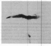
Be absorber 50 µm  $(\varepsilon \ge 2 \text{ kev})$ . The printing of the photo is light enough to show an intense localized source which is embedded in the broad source of softer X-rays on the electrode axis.
