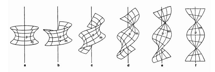
The catenoid is the most characteristic form of the minimal surface of negative curvature. A cross section made with a plane perpendicular to its axis generates a circle. A cross section which contains the axis produces a catenary curve—the so-called hanging chain. If we generate a soap bubble between two parallel rings, the resulting surface of the soap bubble will be the catenoid.
