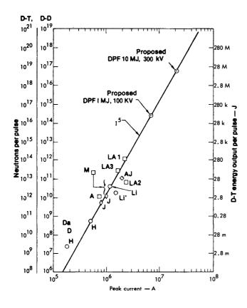
ment program to pay for such a program. Figure 21, which is taken from a Lawrence Livermore Laboratory design study, indicates that a "breakeven" machine of the type designed will occur at about 4 megajoules and 16 megamperes.
