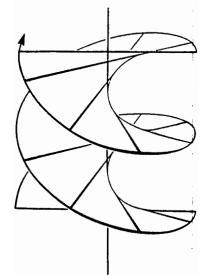
The helicoid is like a spiral staircase and generated by a rotating line that also moves along its axis of rotation. It determines helices of decreasing slope as one moves away from the central axis of the "staircase," and circles are generated. At a zero radius, the intersection becomes a helix of infinite slope, i.e., it becomes the axis of the cylinder.
