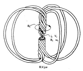
In this diagram of a plasma nodule, a toroidal solenoid wound with a force-free wire carrying current density j, vorticity  $\omega$ , magnetic field B, and mass velocity V.
