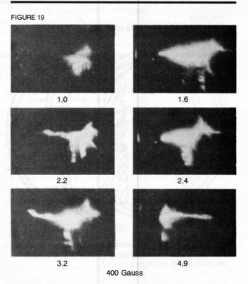
Plasma camera photographs at 0.1 microsecond exposure of the electron density distribution of a copper plasma taken at various times after the gun fires. Plasma, injected from the right, is seen at times of 1.0, 1.6, 2.2, 2.4, 3.2 and 4.9 microseconds as it moves across a 400 Gauss field. The protuberances extend in the velocity cross magnetic field (VXB) direction, downward here. The gun is in opposing polarity.
