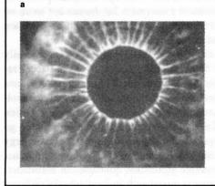
a) The Dense Plasma Focus plasma annulus formed between the plasma focus electrodes.
