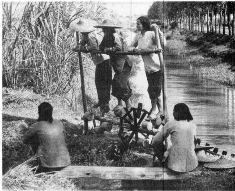
Chinese peasants today are using the same primitive treadle-operated chain pumps to raise water for irrigation that can be seen in a woodcut from 1637.
