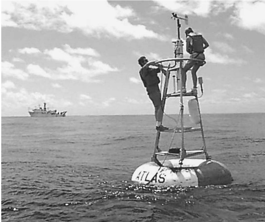
Scientists working on a Tropical Atmosphere Ocean (TAO) Array mooring. There are 65 such buoys along the equator, from the Galapagos Islands to New Guinea. They measure wind and water temperatures, rain, and solar radiation, and transmit the data to the United States via satellite.
