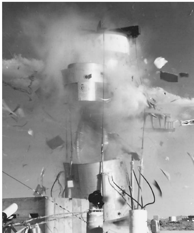
The first laser lethality test of the vulnerability of liquid propellant ballistic missile systems, was conducted for the SDI on Sept. 6, 1985, at the White Sands Missile Range, New Mexico.
