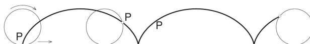
(b) The cycloid is the curve traced out by a point on a circle, as the circle rolls along a line.
