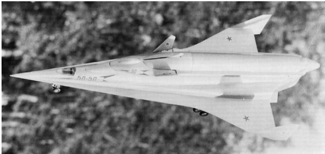
The Soviet "Spiral" aerospace plane, which included a hypersonic airplane booster and small orbital plane on top.
