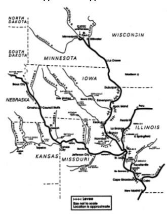
The U.S. Army Corps of Engineers flood-control levee system is extensive for the Lower Mississippi (left), and completely prevented flooding and damage in that region in the huge Flood of 1993. But on the Upper Mississippi (right), such Army Corps infrastructure was never funded and remains to be built; it is there that the 1993 flood caused casualties and devastated towns, industry, and farmlands.
