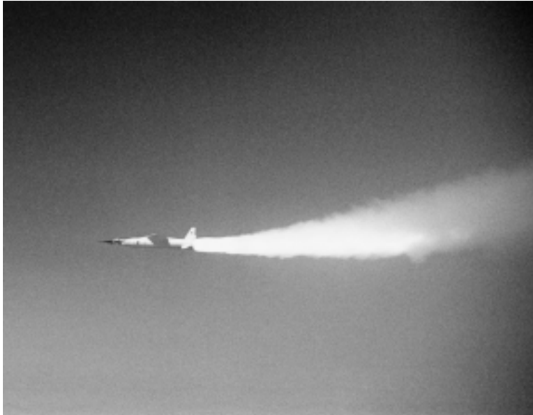
This shows a Pegasus rocket boosting the X-43A scramjet up to speed for the most recent Nov. 16, 2004 test of the scramjet, in which it maintained a speed of 6,600 miles per hour, a record for an air-breathing engine. "I pushed" scramjet development "because this is absolutely necessary for any intelligent approach to space which meets the needs of humanity back here on Earth," said LaRouche.
