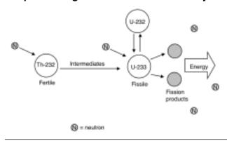
The neutron trigger to start the thorium cycle can come from the fissioning of conventional nuclear fuels (uranium or plutonium) or an accelerator. When neutrons hit the fertile thorium-232 it decays to the fissile U-233 plus fission fragments (lighter elements) and more neutrons. (Not shown is the short-lived intermediate stage of protactinium-233.)
