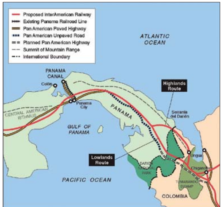
FIGURE 4 Proposed Route Options for the InterAmerican Railway Through the Darien Gap of Panama
