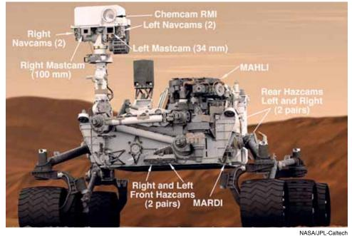
The Curiosity rover points the way to a renaissance of scientific and technological discovery. This graphic shows the location of Curiosity's 17 cameras, which are already sending back to Earth images that are transforming our understanding of Mars.
