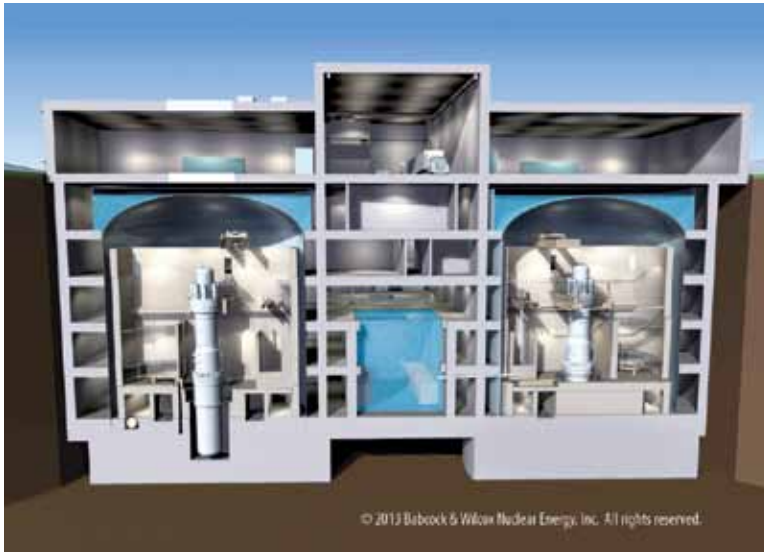
Conceptual drawing of an underground containment structure housing two Babcock & Wilcox mPower reactor modules. On the right is a single mPower reactor, showing the scale of the structure.
