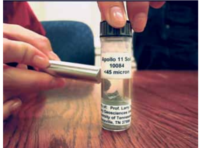
FIGURE 10 Particles of Nano-Phase Elemental Iron Suspended in the Lunar Glass with a Magnet
