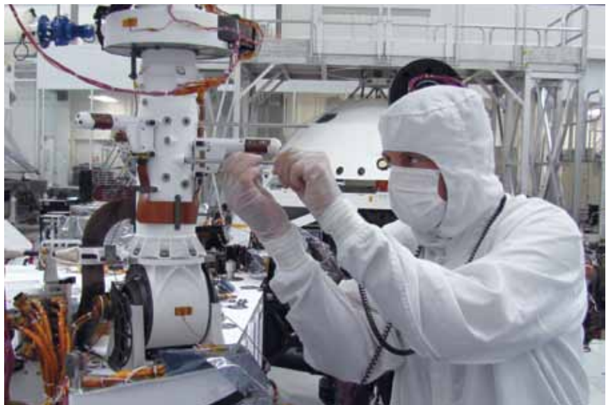
A NASA scientist calibrates two finger-like mini-booms on the Mars rover Curiosity, in preparation for its voyage. It landed on Mars in August 2012.
