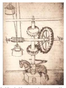
This hoist for lifting building materials was invented by Brunelleschi so the dome could be built, contributing to the successful implementation of Brunelleschi's advances in physical science.
