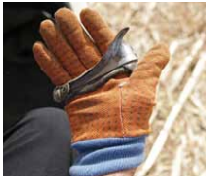
An old handheld device to aid picking a single ear of corn off the stalk.
