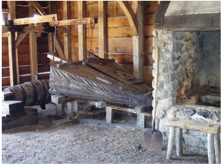
Reconstructed forge with bellows of the Saugus Iron Works, dating from the 1600s in the colonial era in Massachusetts.
