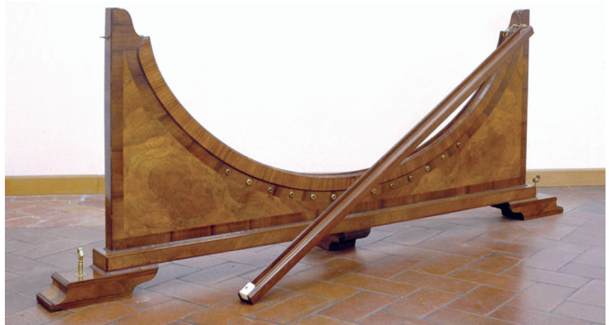
A ball rolling down the pictured cycloid curve will always arrive at the bottom before a ball rolling down a straight path.
