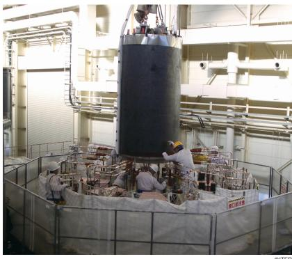
The success of the new world credit system discussed here requires a primary emphasis on nuclear fission and fusion technologies. Shown here, a test coil being built for the ITER poloidal field coil, at the Naka Fusion Institute in Japan, January 2008.
