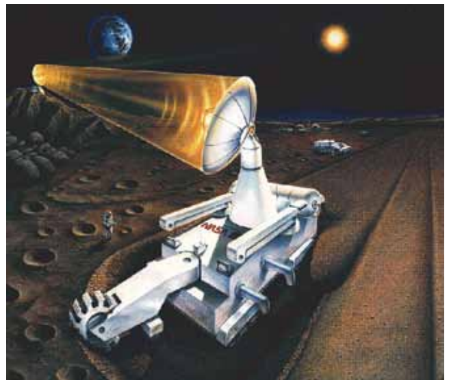
Design concept for a robot to extract helium-3 from the lunar soil.
