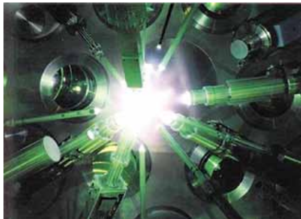
This past June, the National Ignition Facility, part of California's Lawrence Livermore National Laboratory, reported that it had produced 19 quadrillion fusion neutrons in a test shot using a deuterium/tritium capsule. Fifty kilojoules of energy was released, bringing the plasma to within only one order of magnitude of what will be required to reach ignition and breakeven.
