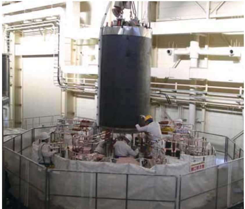
The success of the new world credit system discussed here requires a primary emphasis on nuclear fission and fusion technologies. Shown here, a test coil being built for the ITER poloidal field coil, at the Naka Fusion Institute in Japan, January 2008.
