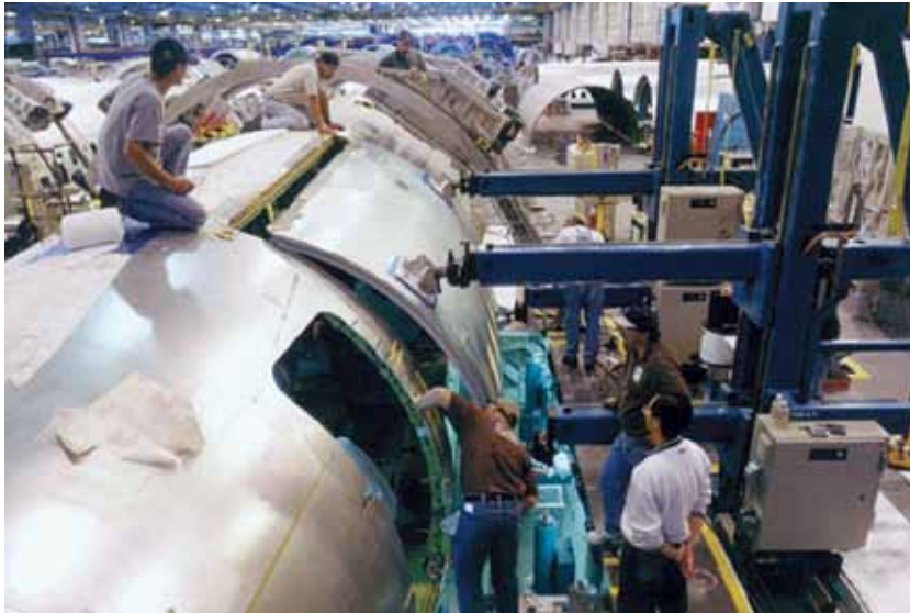
Workers installing the main-deck cargo door on a 737-700C at Boeing's Plant #2 in Wichita, Kansas.
